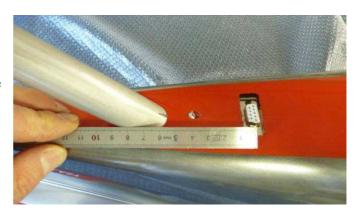
Insert the electric wiring in the fuselage. The wiring must be secured to the fuselage and protected against the engine heat (tailpipe and turbine).
