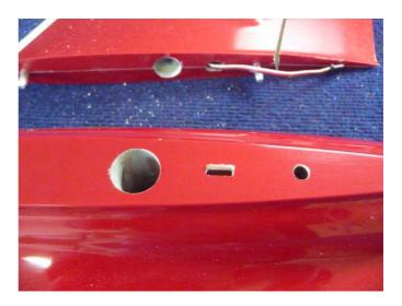
Cut a large hole in the rudder root for the electric wiring.
