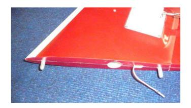
Put the servo cover on the stabs. Drill 4 holes 1 mm diameter in the stab for the screws.
