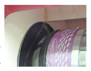
Adjust the position of the engine / beginning of the exhaust tube so the engine exhaust enter for about **20 mm** in the aluminium inlet.
