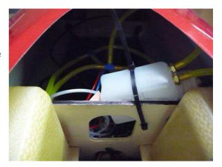
The fuel tank will be attached to the fuel tank plywood frame with plastic T rap.
