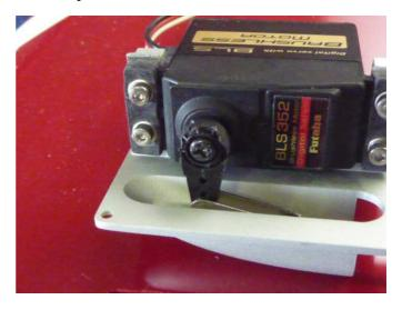
Use a plastic servo control horn. The steel link will be at 14 mm from the servo axis.
