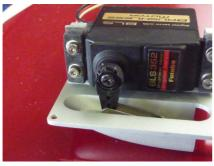
Put the 2 servo covers on the wing. Drill 8 holes 1 mm diameter in the wing for the screws.
