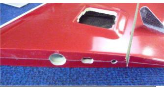
Glue the 2 aluminium pins in the stab with cyano. Pins must overtake for about 10 mm.
