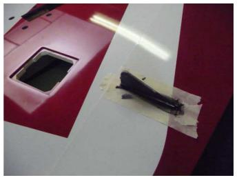
Drill a large hole in the wing root for the electric wiring and gear tubing.
