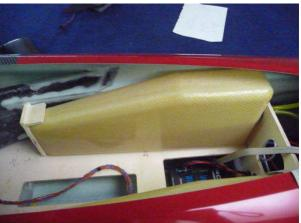
Insert the rear plywood frame to secure the rear of the tanks. Glue it with quick epoxy.
