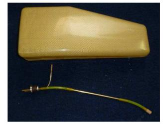
Insert the fuels tanks in the fuselage against the front plywood frame.
